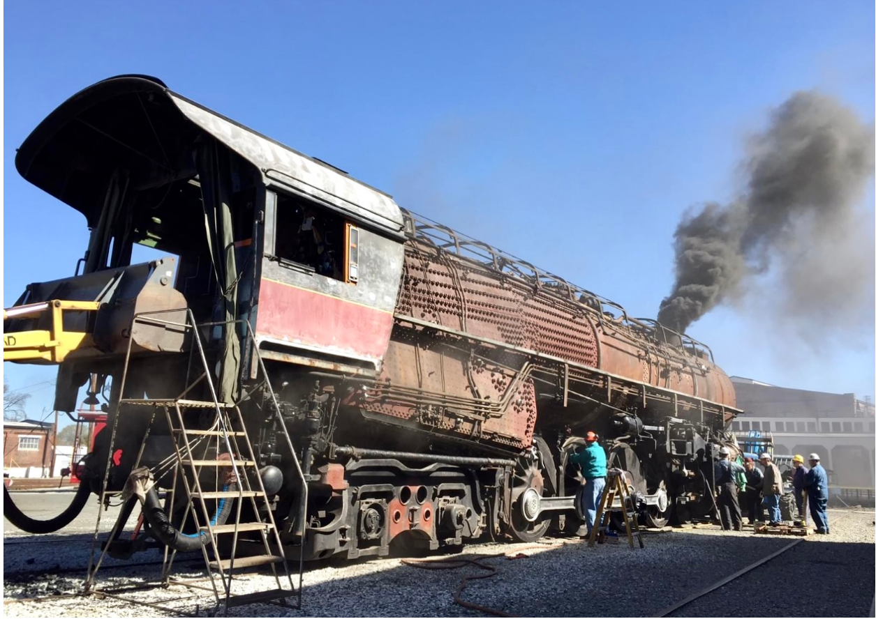
Photo 5: 611 test fire during restoration April 2015. Photo: Virginia Museum of Transportation
